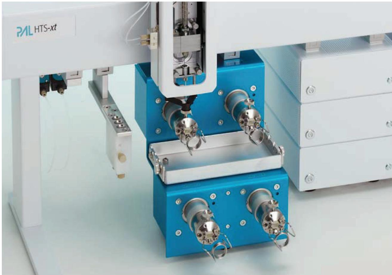
PAL HTS-xt equipped with 4-fold valve Drive
